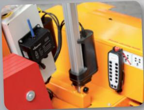
If desired, a cordless remote control can be selected, which also makes all motion functions accessible.
