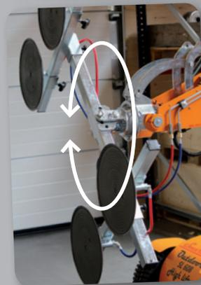
*The electrical rotation of the yoke makes it easier to handle heavy items.*
