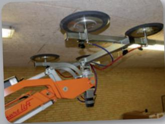
The SmartLift can lift items horizontally in rooms with low ceiling height.
