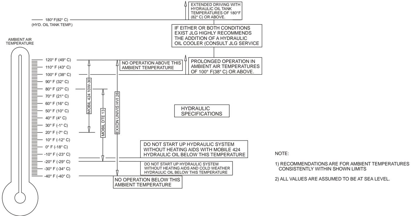
**Figure 6-5. Engine Operating Temperature Specifications - GM - Sheet 2 of 2**
