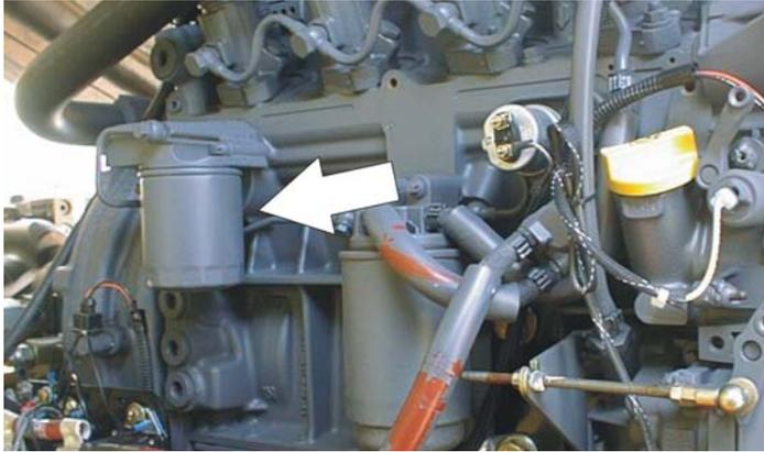
Lube Point(s) - Fill Cap/Spin-on Element
