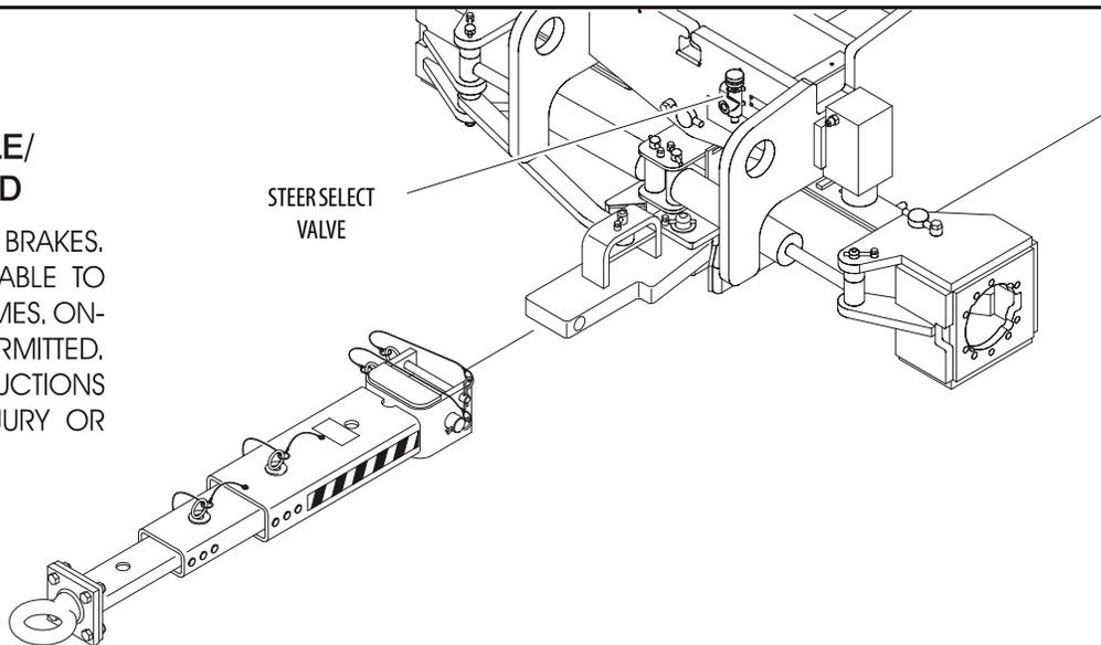
**Figure 4-4. Towbar Connecting Points**
