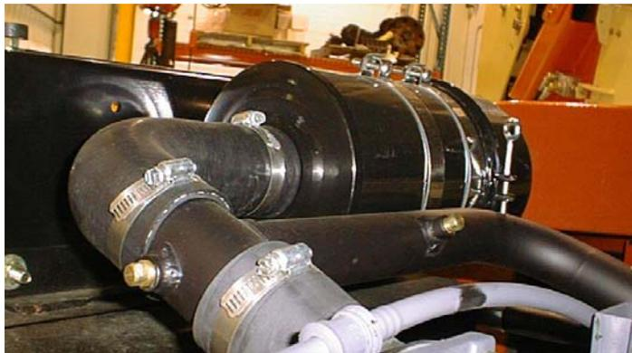
Lube Point(s) - Replaceable Element
