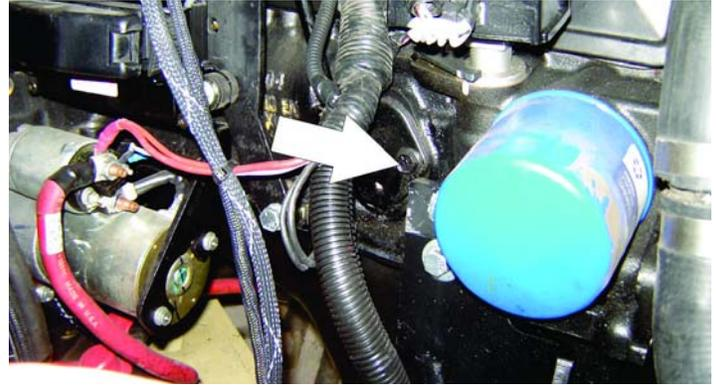
Lube Point(s) - Fill Cap/Spin-on Element
