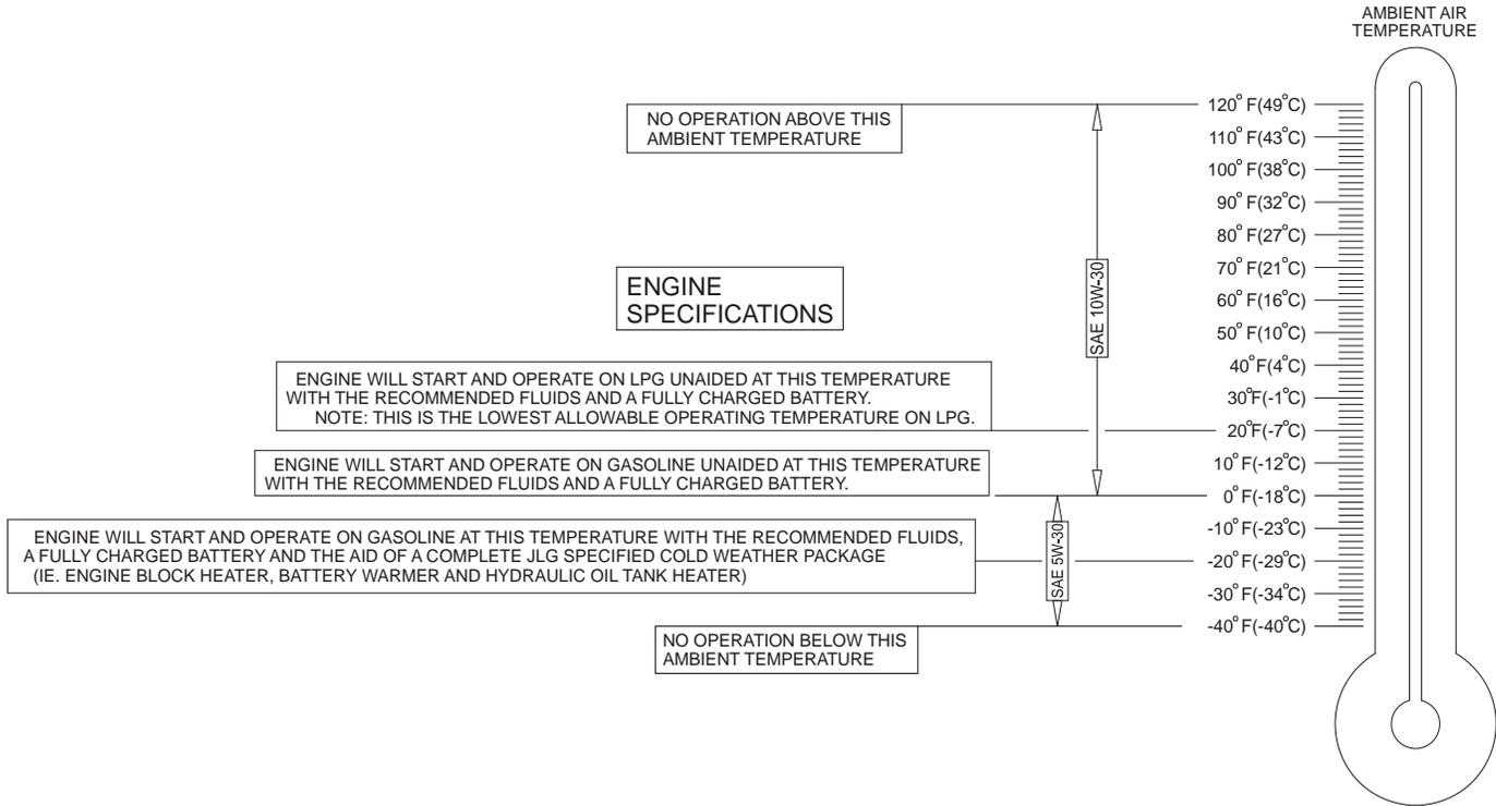
Figure 6-4. Engine Operating Temperature Specifications - GM - Sheet 1 of 2
