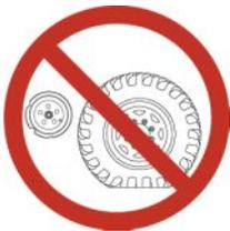
**DO NOT** use the MEWP when the wheels or tires are damaged (refer to [Section 4.2-7](#)).
