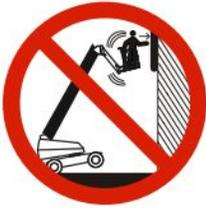
**DO NOT** exceed the maximum side force on the platform capacity label when elevated (refer to [Section 7.7](#)).
