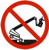
**DO NOT** drive elevated near depressions or holes of any type, loading docks, debris, drop-offs or surfaces that may affect the stability of the MEWP. IF OPERATION IN AREAS WITH HOLES OR DROP-OFFS IS ABSOLUTELY NECESSARY, elevated driving shall not be allowed. Position the MEWP horizontally only with the platform fully-lowered. After ensuring that all 4 wheels have contact with a firm, level surface, the platform can be raised. After elevation, the drive function must not be activated.
