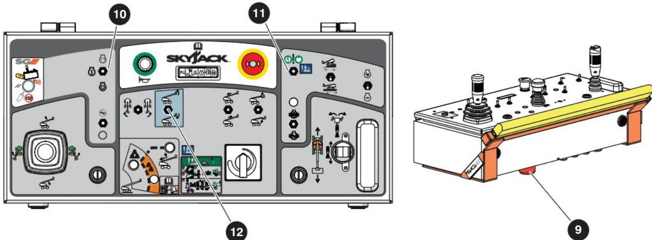
14. Press the **sensor bar** for less than 1 second and then release it.
