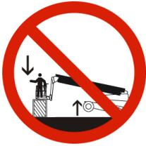
**DO NOT** use the boom to push or pull other objects, or to lift the chassis.
