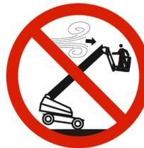
**DO NOT** raise the platform or operate elevated in windy or gusty conditions that exceed the limits specified in [Section 7.7](#).
