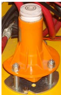
Figure 4-11. Level Sensor Pendulum Based
