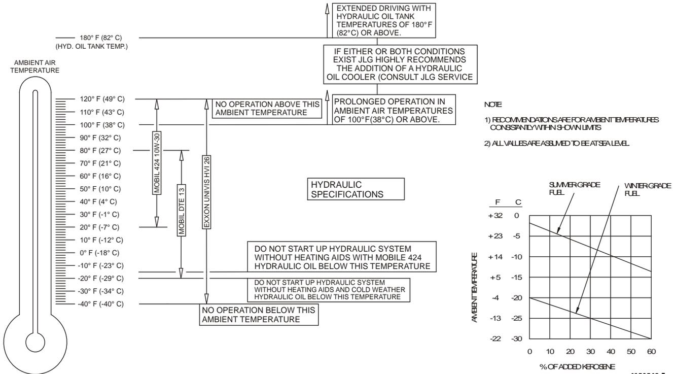
Figure 6-2. Engine Operating Temperature Specifications - Deutz - Sheet 2 of 2
