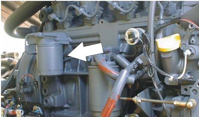
Lube Point(s) - Fill Cap/Spin-on Element
