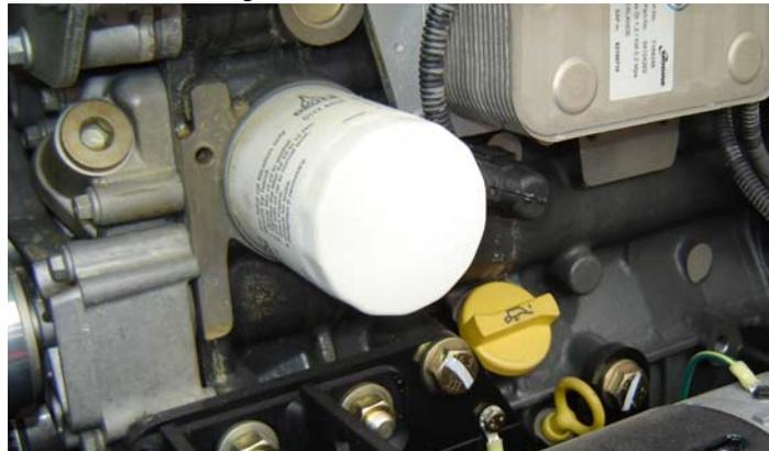
Lube Point(s) - Fill Cap/Spin-on Element
