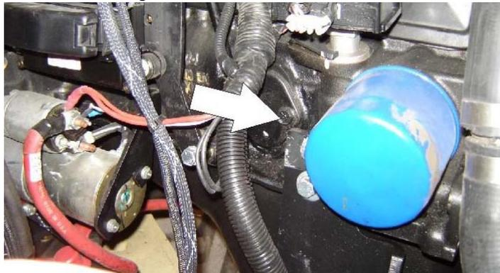
Lube Point(s) - Fill Cap/Spin-on Element
