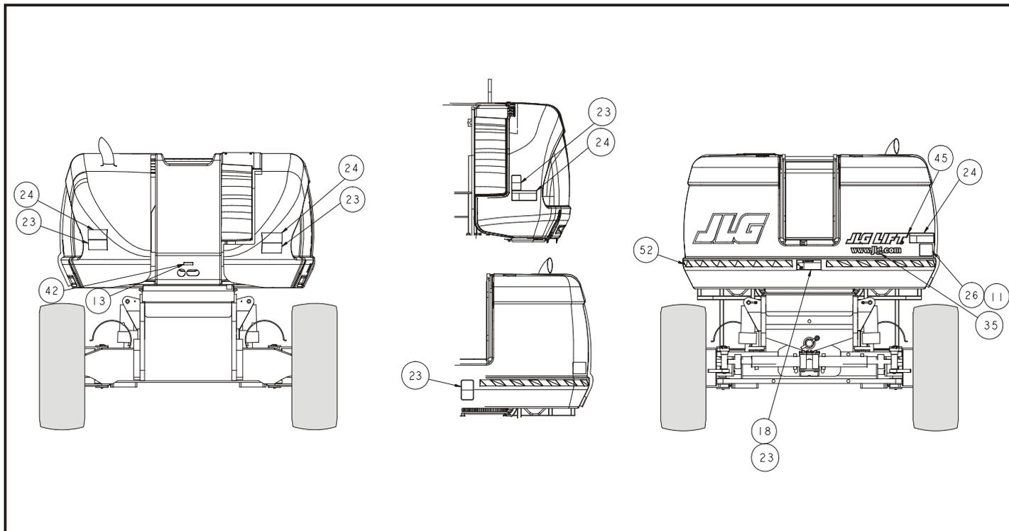
Figure 4-10. Decal Installation - Sheet 3 of 5
