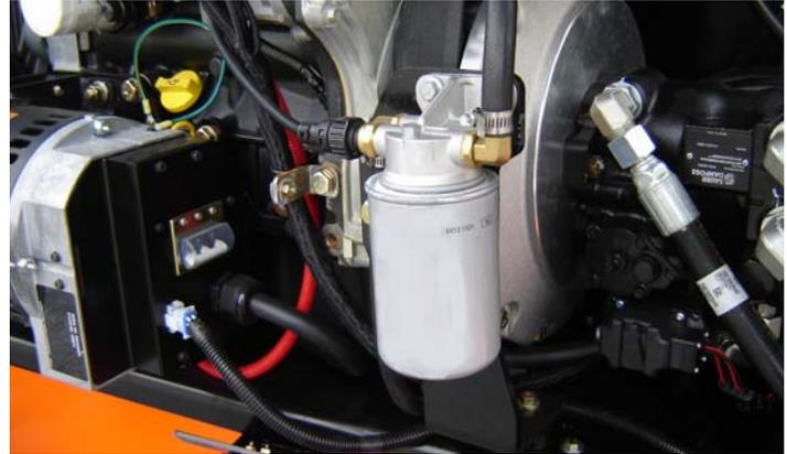
Lube Point(s) - Replaceable Element
