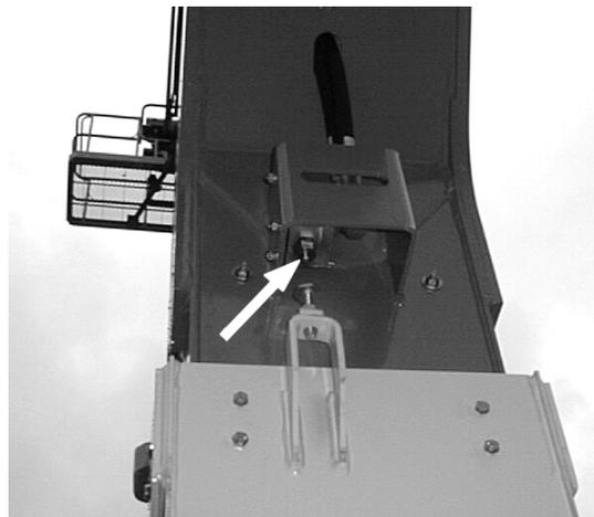
**Figure 2-6. Tower Boom Horizontal Limit Switch**
