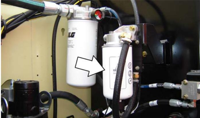
Lube Point(s) - Replaceable Element
