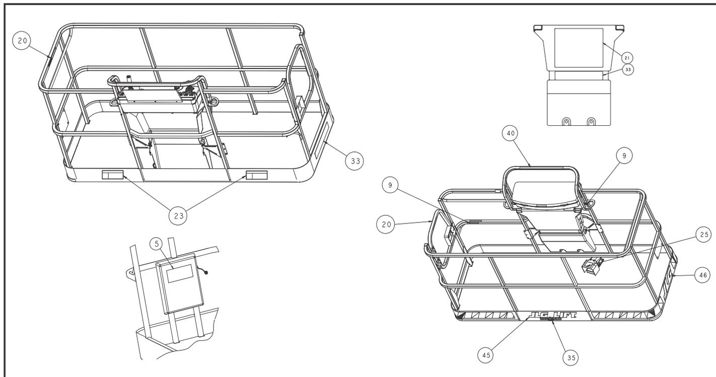
Figure 4-12. Decal Installation - Sheet 5 of 5
