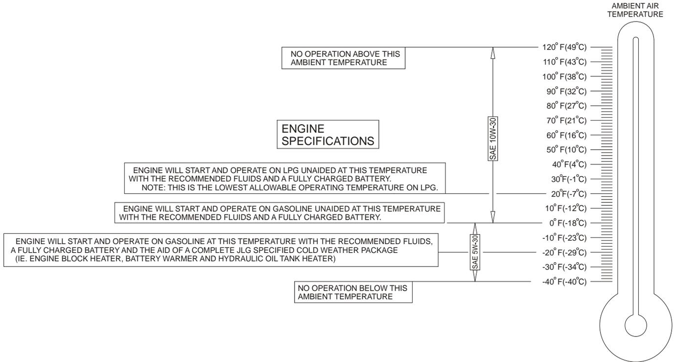
**Figure 6-3. Engine Operating Temperature Specifications - GM - Sheet 1 of 2**
