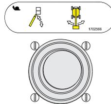
**NOTE:** Main boom lift and swing functions may be selected in combination. Maximum speed is reduced when multiple functions are selected.
