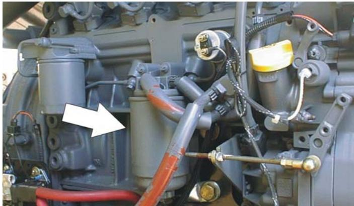
Lube Point(s) - Replaceable Element
