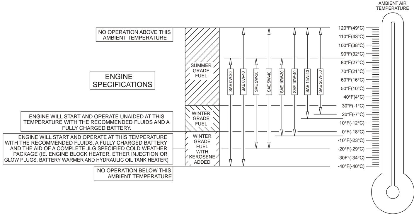
**Figure 6-1. Engine Operating Temperature Specifications - Deutz - Sheet 1 of 2**
