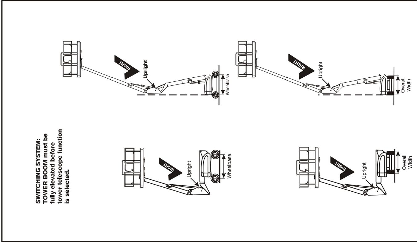
Figure 4-5. Boom Upright Positioning - Sheet 1 of 2
