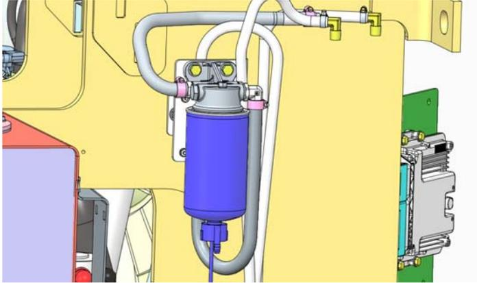
Lube Point(s) - Replaceable Element
