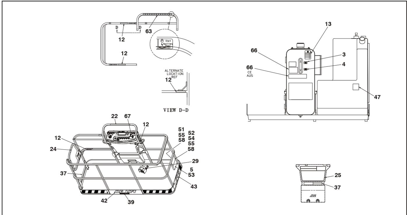
Figure 4-12. 600A & 600AJ Decal Installation - Sheet 3 of 4
