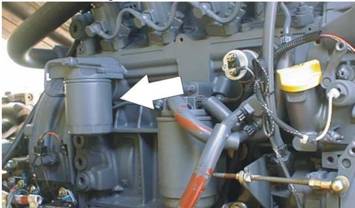
Lube Point(s) - Fill Cap/Spin-on Element
