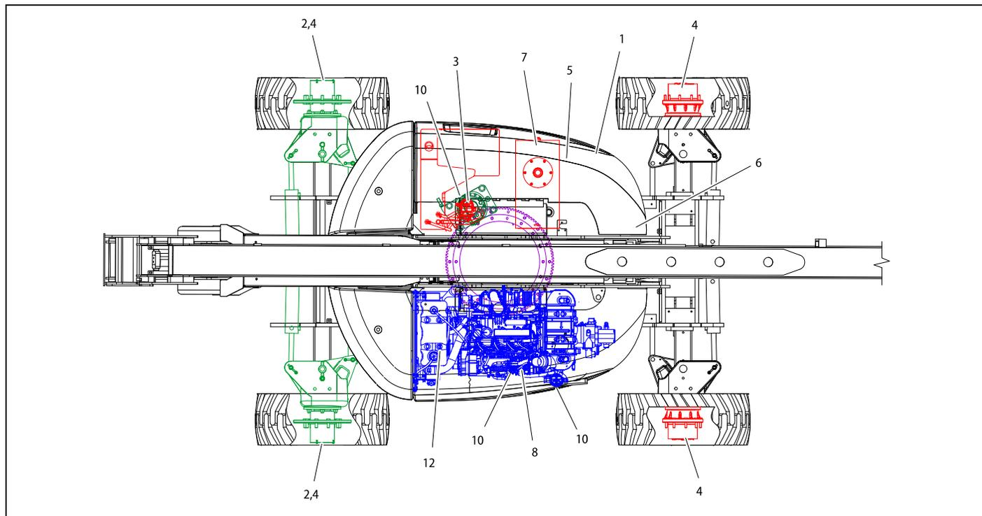
**Figure 6-7. Operator Maintenance & Lubrication Diagram - Deutz TD2.9**
