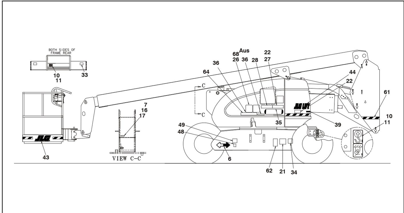
Figure 4-10. 600A & 600AJ Decal Installation - Sheet 1 of 4
