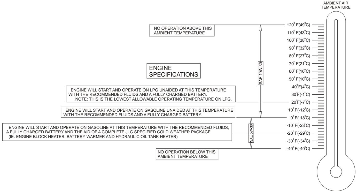
**Figure 6-4. Engine Operating Temperature Specifications - GM - Sheet 1 of 2**
