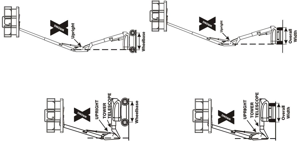
Figure 4-6. Boom Upright Positioning - Sheet 2 of 2
