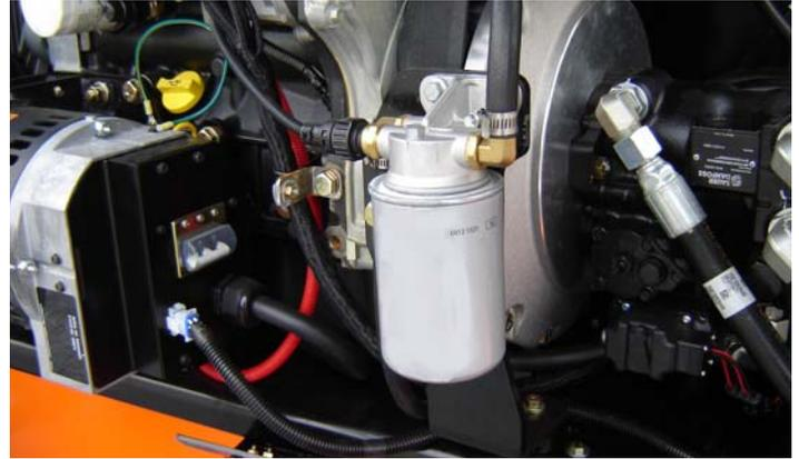
Lube Point(s) - Replaceable Element
