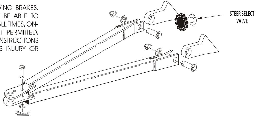
**Figure 4-7. Towbar Connecting Points**
