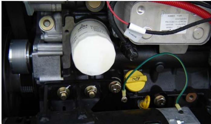
Lube Point(s) - Fill Cap/Spin-on Element
