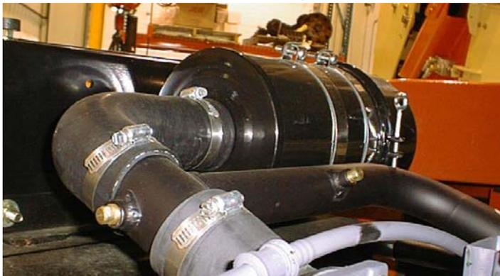
Lube Point(s) - Replaceable Element
