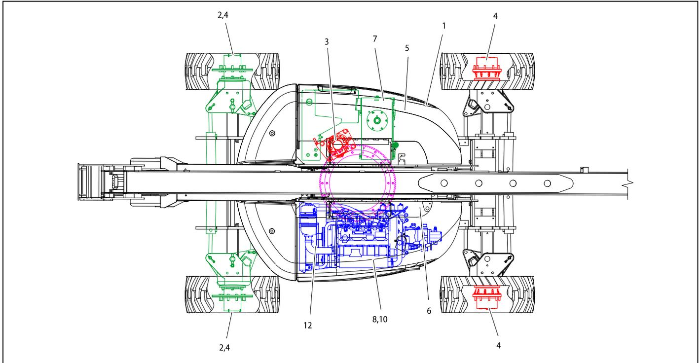
**Figure 6-6. Operator Maintenance & Lubrication Diagram - Deutz D2011L04**
