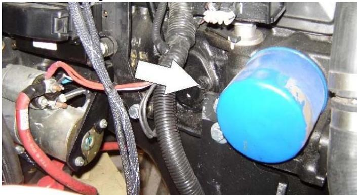
Lube Point(s) - Fill Cap/Spin-on Element
