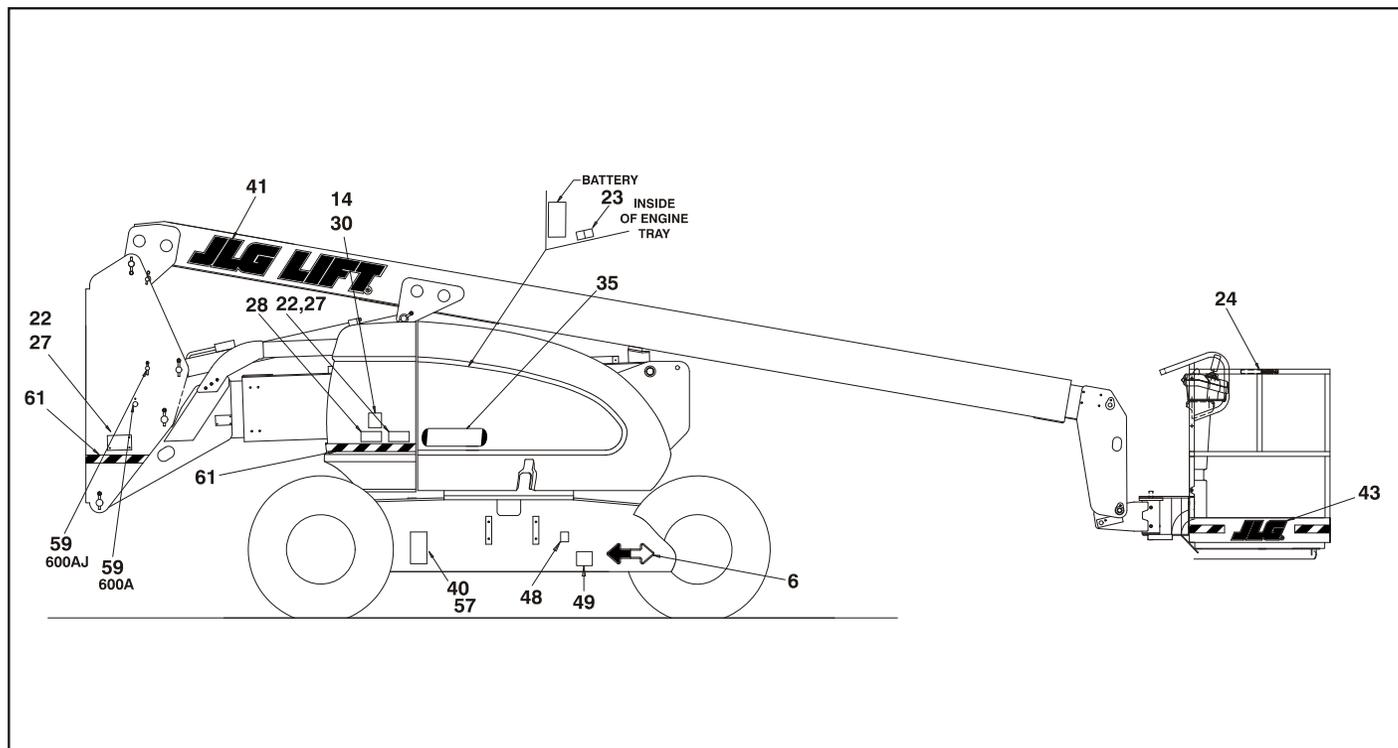
Figure 4-11. 600A & 600AJ Decal Installation - Sheet 2 of 4
